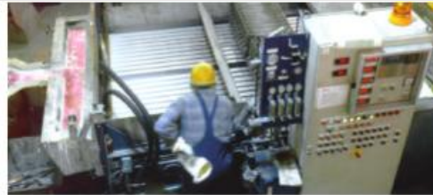
Figure 2. View of feed to horizontal continuous caster Foto: HERTWICH ENGINEERING, Brunnau-AUSTRIA
