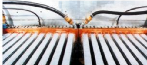
Figure 3. View of cast bars emerging from caster. Twenty strands are cast from two molds
